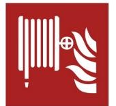
Sign marking a fire hose, consisting of fire protection sign F002
