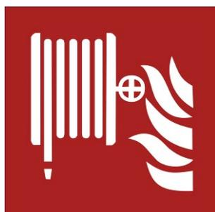
Sign marking a fire hose, consisting of fire protection sign F002
