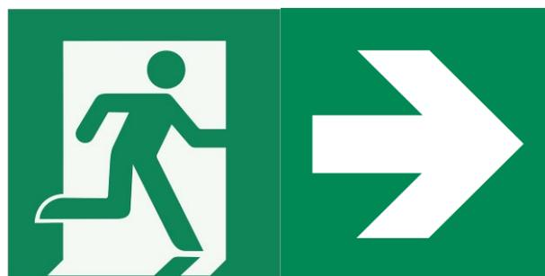
Sign marking an escape route/emergency exit, consisting of emergency sign E002 "Emergency Exit" and supplementary sign (directional arrow) (sample)
